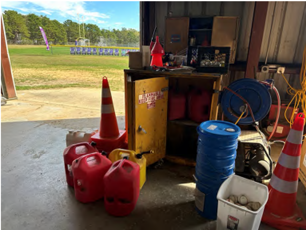
Photo 20: Flammables cabinet with gasoline storage in maintenance garage.
