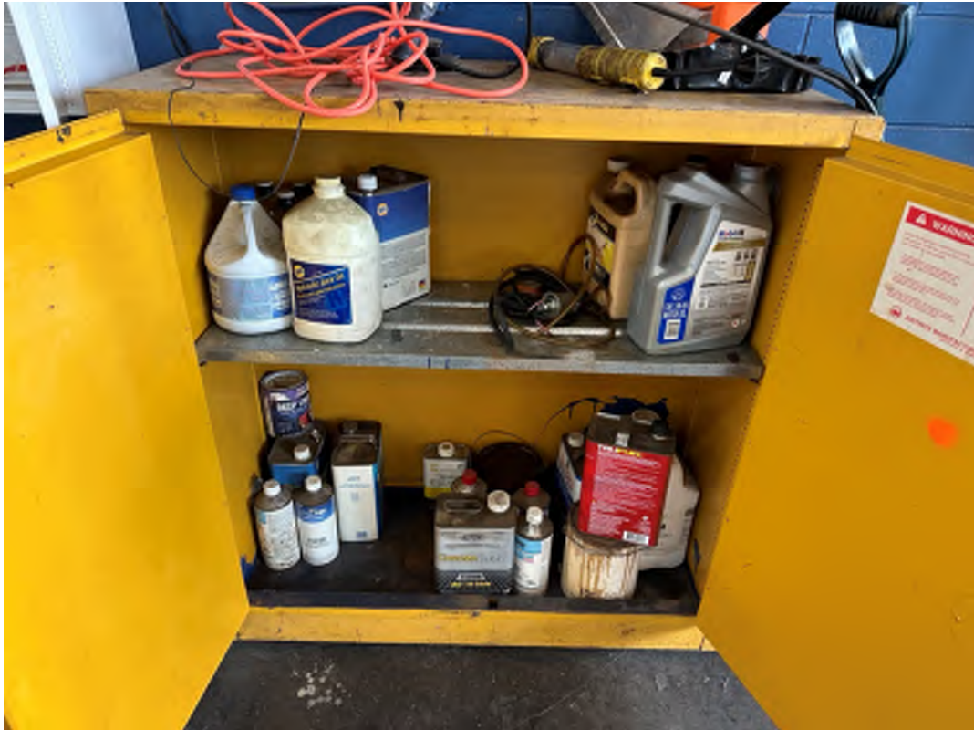
Photo 5: Flammables cabinet with oil and lubricant storage in automotive shop.
